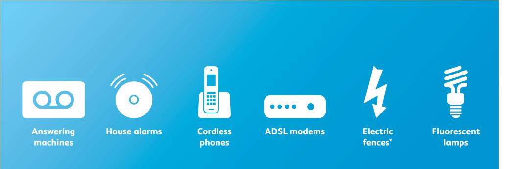
\*Faulty electric fences can cause impulse noise on the ADSL line which may prevent the ASDL line from syncing. Check for any arcing (electrical breakdown) from the fence due to faulty/cracked isolators, plants or any foreign objects touching the fence.
